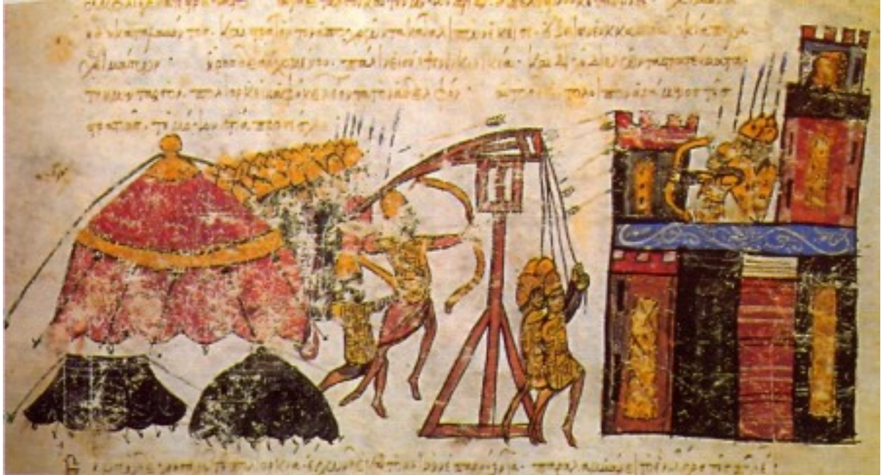
Figure 3 Byzantine manuscript depicting a traction trebuchet in siege of a fortification. Note the similarity to the design to the engine in figure 2. It is possible that the Byzantines were using these weapons by the late 500's.
