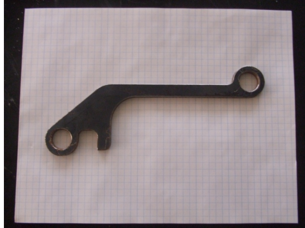
Figure 8 Trigger fabricated for our Trebuchet (5mm squares)
